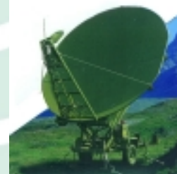
Ground Based Radar
