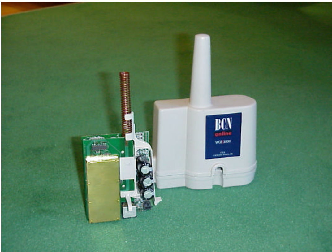
Figure 4: Photograph of Gas meter transmitter unit
